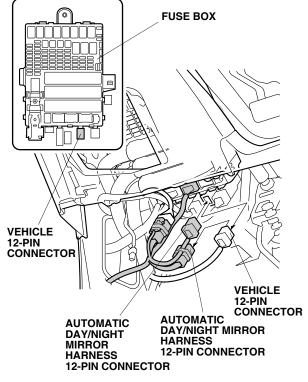
23. Secure the automatic day/night mirror harness to the vehicle harness with one wire tie.
