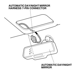
30. Align the green tape on the automatic day/night mirror harness with the edge of the headliner. Route the automatic day/night mirror harness through the grooves in the harness cover. Secure the harness cover to the mirror stay.
