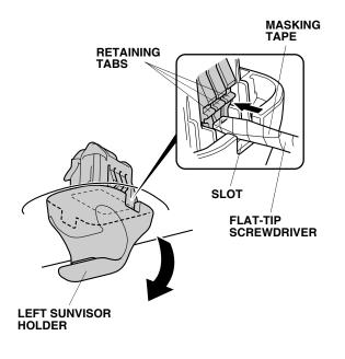
10. Use a flat-tip screwdriver wrapped with masking tape to release the three retaining tabs on the other side of the left sunvisor holder. Remove the holder.
